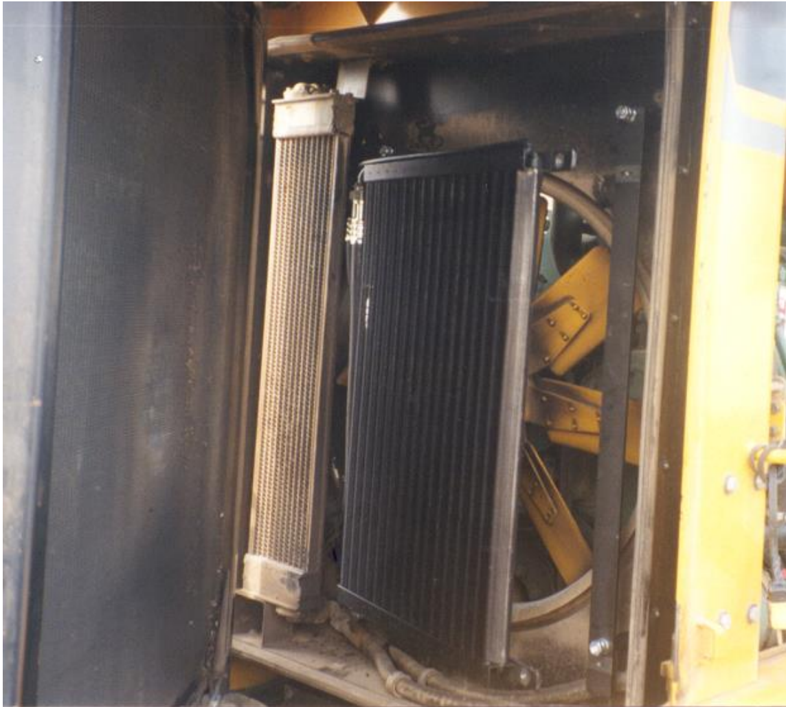
Condenser view showing mount points and fitting arrangement.
