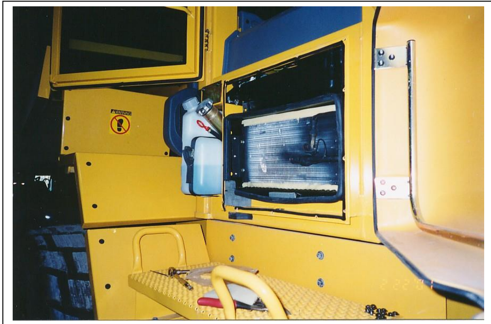
Face on view of evaporator with hoses and thermostat probe.
